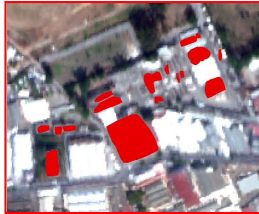
Fig. 3b. A-c roofing in the area of S. Basilio (below in the image).
