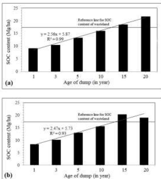
**Fig. 8** Temporal changes in total SOC content of dumps and backfilled areas for (a) 0-15cm and (b) 15-30 cm depth.
