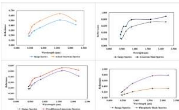
**Fig. 7** Spectral reflectance plots showing reflectance values of reference spectra (USGS) along with image spectra for various materials as identified using the SAM algorithm
