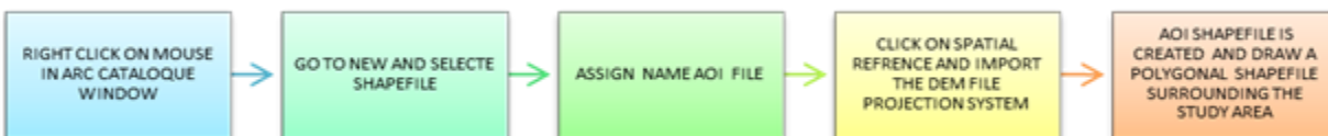
Module.4- processes of creating a new shape file with accurate UTM Projection Data
