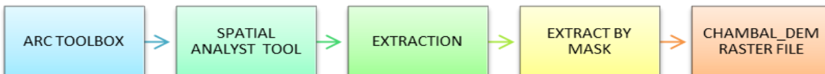
Module.5. processes of Extraction of Chambal study area by Extraction of Mask
